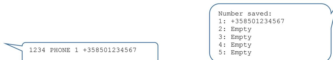
The diagram shows two speech bubbles representing an SMS. The left bubble contains the command: `1234 PHONE 1 +358501234567`. The right bubble contains the response: `Number saved:`, `1: +358501234567`, `2: Empty`, `3: Empty`, `4: Empty`, and `5: Empty`.
