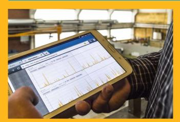
Energy and utility monitoring was the original approach of Apollo asset monitoring. Manual reading walks were replaced by more frequent and exact remote reading.
